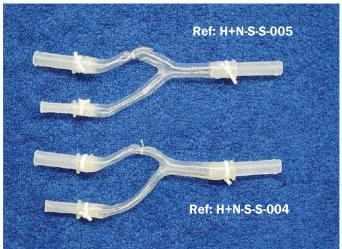
ELASTRAT replicas are compatible with modern imaging modalities such as digital subtraction angiography, computed tomography and magnetic resonance imaging. Providing the use of an adequate circulating fluid, Doppler techniques can also be performed. The in vitro models transparency to light makes them suitable for video and photographic monitoring.
