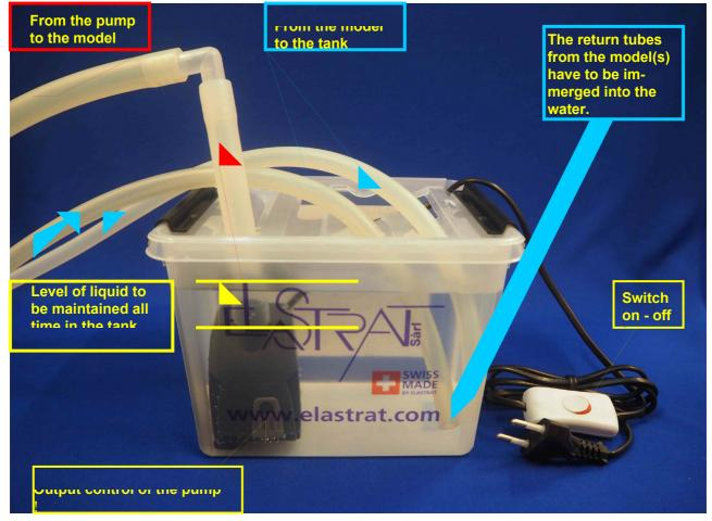
Tank specially developed with holes to hold the tubes and have the pump immersed in water **Size of tank: 14 x 20 cm height.** Details of 110 and 220 Volts aquarium continuous flow pumps:
