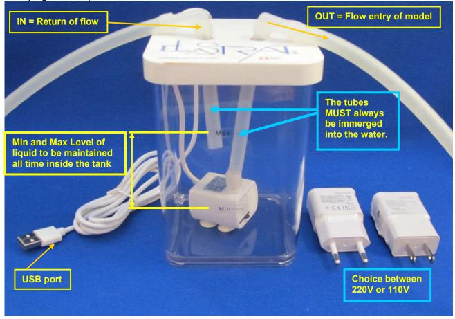
In use with a "Specific patient" Head model. Tank size: 9 x 9 x 14 cm height, max capacity 1 lt.
