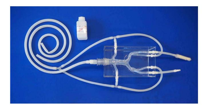
ELASTRAT's in vitro models respect human anatomy and are designed for the development and demonstration of stents, coïls and catheters.
