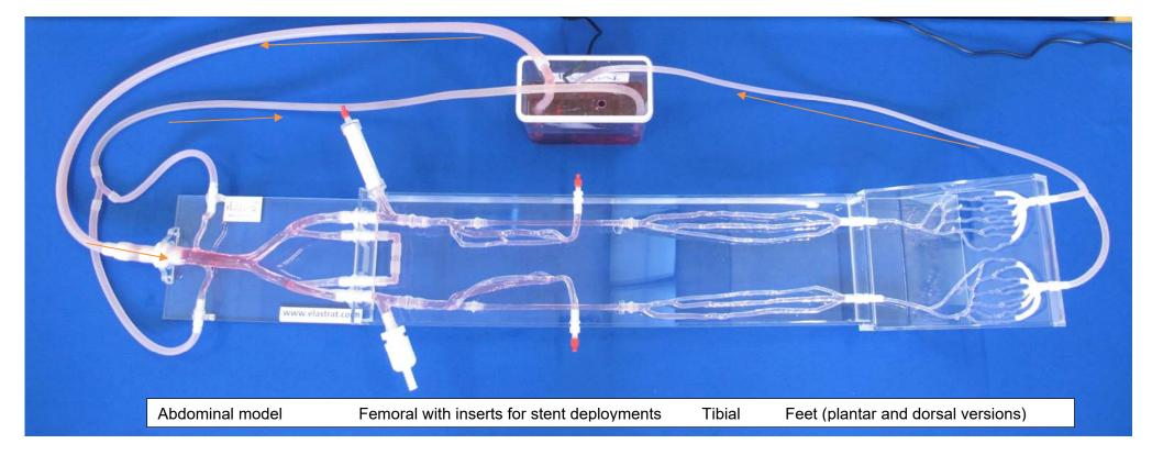
This model is made to work in a closed water circuit with a continuous flow or a pulsatile pump. A heather can also be added.
