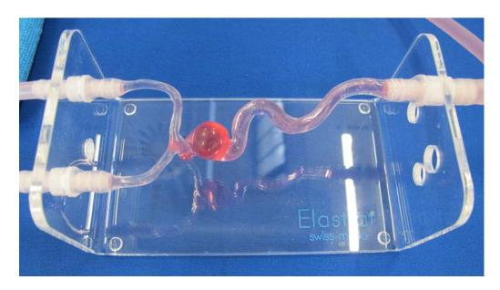
Ready to work in a closed water circuit with a 1L tank and a continuous flow pump. A peristaltic pump can also easily be plugged to this model.
