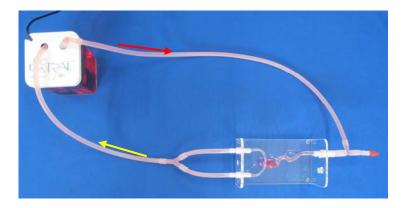
ELASTRAT in vitro models respect human anatomy and are designed for the development and demonstration of stents, coïls and catheters. They provide a realistic environment for the simulation of endovascular procedures, pre-surgery training, studies, and teaching purposes for interventionists.
