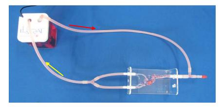
ELASTRAT in vitro models respect human anatomy and are designed for the development and demonstration of stents, coïls and catheters. They provide a realistic environment for the simulation of endovascular procedures, pre-surgery training, studies, and teaching purposes for interventionists.
