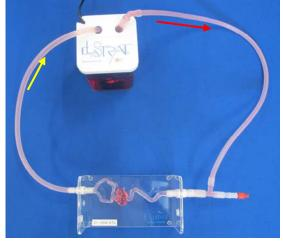
ELASTRAT in vitro models respect human anatomy and are designed for the development and demonstration of stents, coïls and catheters. They provide a realistic environment for the simulation of endovascular procedures, pre-surgery training, studies, and teaching purposes for interventionists.
