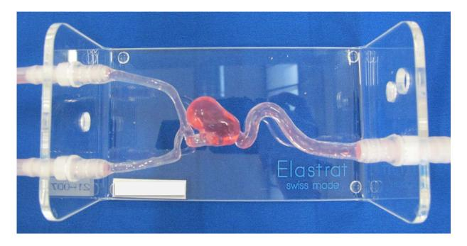
Ready to work in a closed water circuit with a 1L tank and a continuous flow pump. A peristaltic pump can also easily be plugged to this model.
