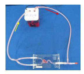
ELASTRAT in vitro models respect human anatomy and are designed for the development and demonstration of stents, coïls and catheters. They provide a realistic environment for the simulation of endovascular procedures, pre-surgery training, studies, and teaching purposes for interventionists.
