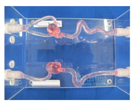
Ready to work in a closed water circuit with a 1L tank and a continuous flow pump. A peristaltic pump can also easily be plugged to this model.
