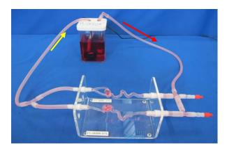
ELASTRAT in vitro models respect human anatomy and are designed for the development and demonstration of stents, coïls and catheters. They provide a realistic environment for the simulation of endovascular procedures, pre-surgery training, studies, and teaching purposes for interventionists.
